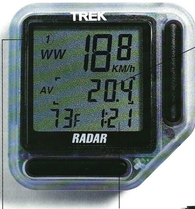
**Workout Window tracks separate data for individual segments of a ride, apart from overall ride averages, with a quick toggle-push on and off. It's great for keeping track of top-performance during high-intensity portions of training rides. All of this is presented in a user friendly format.**
