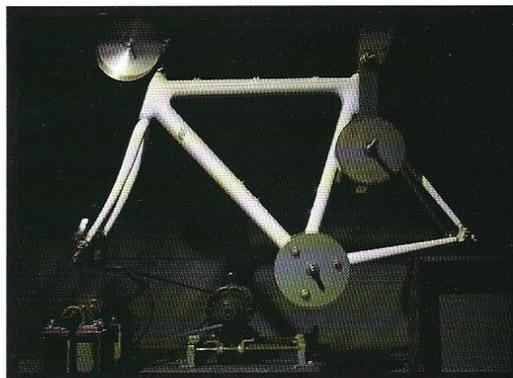
**In the test lab, we subject Trek frames to grueling high-cycle fatigue tests. Our OCLV carbon frames went over a million cycles without failure.**
