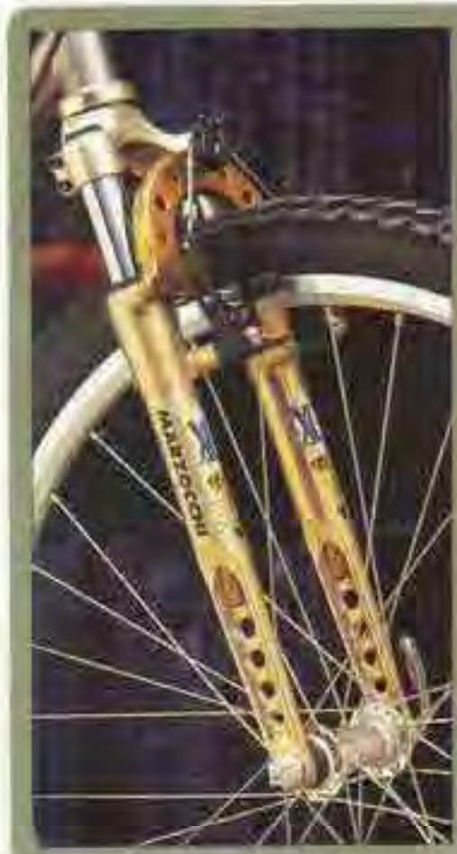
Marzocchi XC 600 Air/Oil Suspension Weight: 2.9 lbs. Travel: 2 inches
