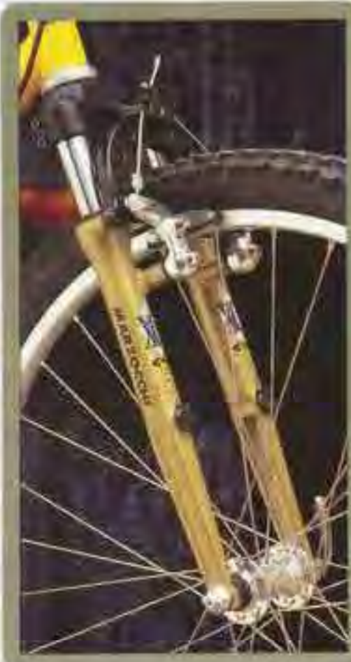
Marzocchi XCR Air/Oil Suspension Weight: 2.7 lbs. Travel: 2 inches
