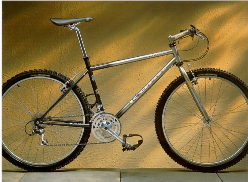
Sugino XP crank: Four Spider design
