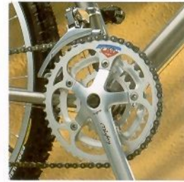
Sugino XP crank: Four Spider design
